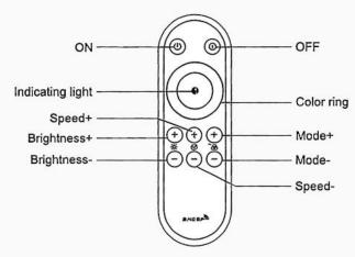
This product adopts wireless RF for communication, through which lights can be remotely controlled over long distance and over obstacles. The remote control uses capacitive sensing touch keys to control the light.
